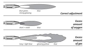
Then adjust a neutral flame. That means that the strong glowing blue-green flame core must be sharply surrounded by a dark blue flame edge (secondary flame).
